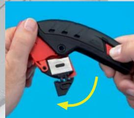
...pull squeeze lever out and continue until it stops. Flip open black blade cover.
