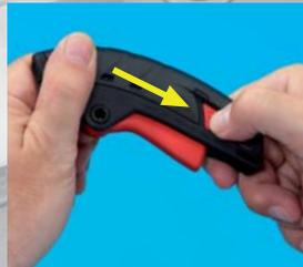
Begin with knife in locked position by pressing . Slide black blade change button toward back of the knife. While depressing this button...
