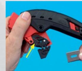
Reverse or replace the blade making sure to locate it on the pin. Close the blade cover...
