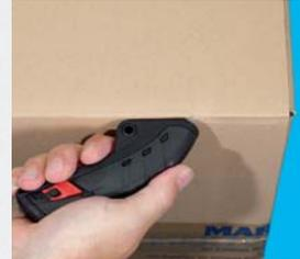
Cut with the blade into the material (e.g. carton). Ensure sufficient pressure is applied when cutting to activate the auto retract mechanism. It will audibly click into place.
